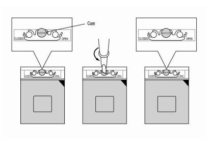
Figure 4-38 Unlocking the CPU
